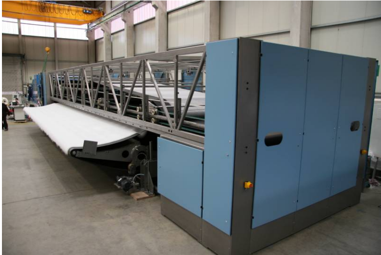
Crosslapper for papermachine clothing applications in 14.5 m working width
